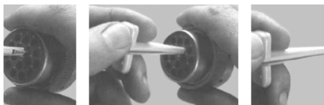
Figure 6-16. HD/HDP Contact Removal
